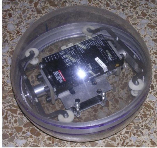
Figure 1.5: A picture of HIT and its internal driving mechanism [12].
